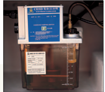
The automatic lubrication pump is installed at low level for easy monitoring.
