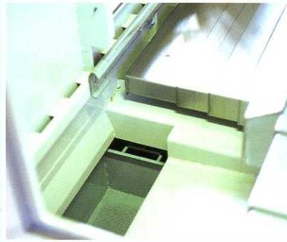
Large outlet for chips and coolant
